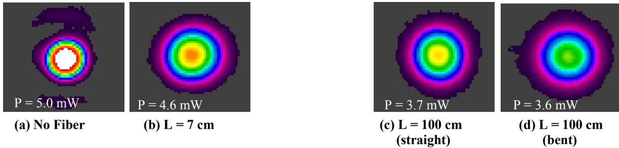
**Figure 5.**  $d = 300 \mu\text{m}$ ,  $\lambda = 9.5 \mu\text{m}$ ,  $2w_o/d = 0.77$ : Two-dimensional beam profile of a QCL operating at  $\lambda = 9.5 \mu\text{m}$  (a) measured 11.5 cm after an  $f = 76 \text{ mm}$  focusing lens and (b) – (d) measured 3.75 cm after exiting  $d = 300 \mu\text{m}$  hollow fibers with two different lengths (bent and straight). The measured power in each case is also displayed.
