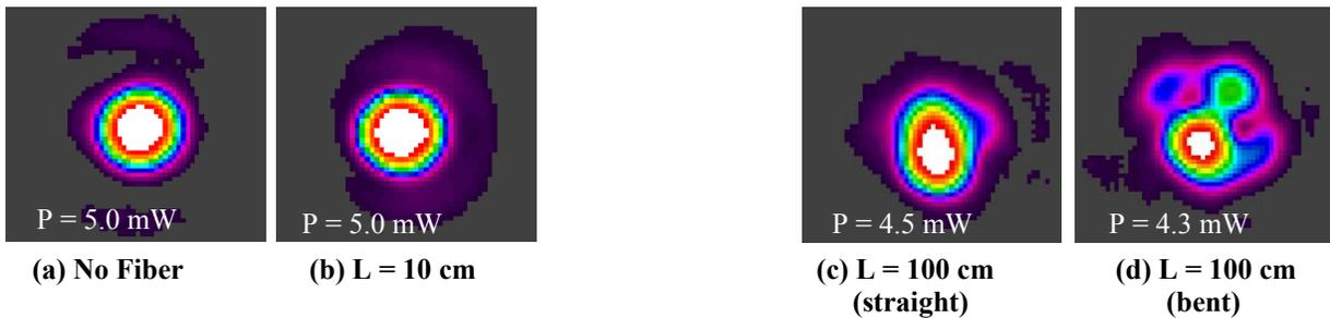
**Figure 6.**  $d = 500 \mu\text{m}$ ;  $\lambda = 9.5 \mu\text{m}$ ;  $2w_o/d = 0.46$ : Two-dimensional beam profile of a QCL operating at  $\lambda = 9.5 \mu\text{m}$  (a) measured 11.5 cm after an  $f = 76 \text{ mm}$  focusing lens and (b) – (d) measured 3.75 cm after exiting  $d = 500 \mu\text{m}$  hollow fibers with two different lengths (bent and straight). The measured power in each case is also displayed.
